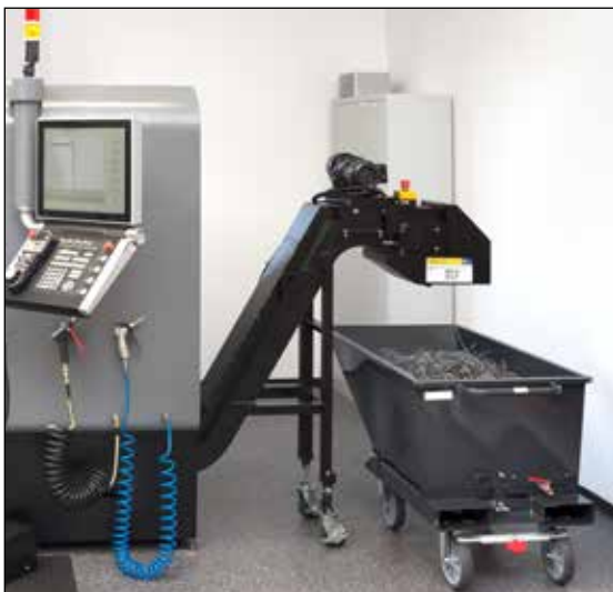
Example of use: Sheet metal dump truck as bin.
